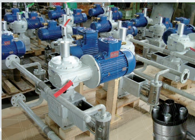
Double acting heads in opposite side
