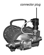
The pressure switch stops the pump once the preset pressure of 3 bar is reached (top switching point). When pressure reaches the lower switching point the pump will start automatically. Switch hysteresis is set to 30% as standard.
