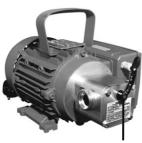
Dry run protection prevents overheating of the impeller. When the pump is running dry and heats up the thermo sensitive switch turns off the motor. After cooling off the pump is ready to use again.
