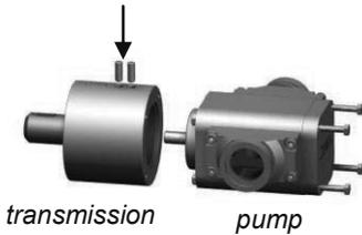
The transmission with 24 mm stainless steel shaft for disc adaption can be used with pump types 2001-A, 2001-B and 2001-C. Pump with transmission is normally delivered as a completely assembled unit.
