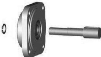
5. Detach locking ring and press out shaft.
