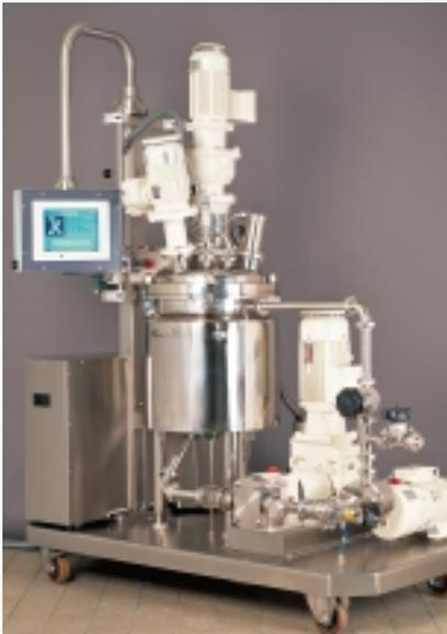
An EMA 100 with most up-to-date process control system with touch screen.
