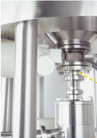
EMA 300 with dispersing machine DR 2000/10 directly connected to the bottom outlet.
