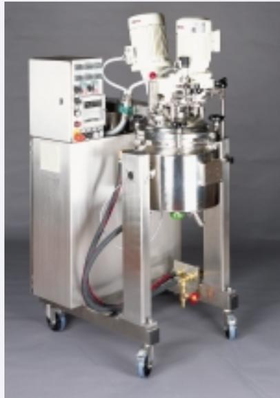
EMA 15 pilot plant with all components necessary to develop creams and emulsions: anchor stirrer, ULTRA-TURRAX®, vessel that can be heated and evacuated as well as electric control.
