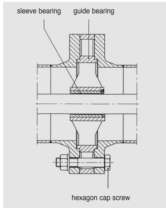
The guide bearings are positioned by centrings in the column shafts and tightened by hexagon cap screws. The sleeve bearing is located in the hub of the guide bearing. Standard bearing material for clean liquids is sintered Graphite-Teflon foil. The bearing foil is of floating design and has dry running capability.
