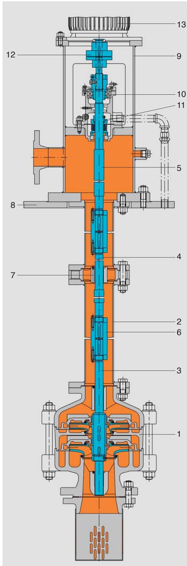
*HZV Barrel-casing Design*
