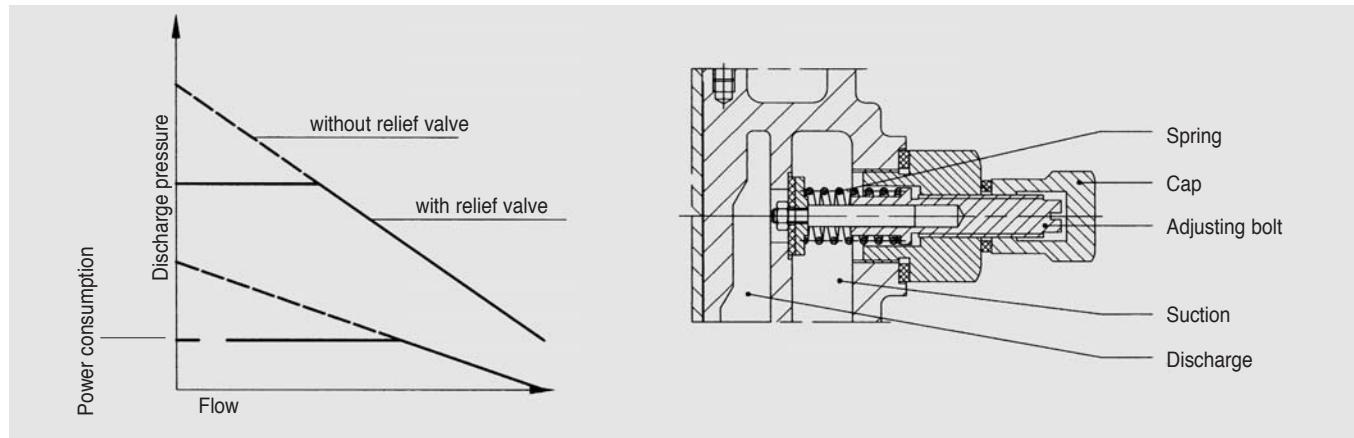
Contrary to centrifugal pumps, the side channel pumps generate a steep head rise and an increased power consumption at lower flow rates. Power consumption and discharge pressure reach the maximum at closed discharge. To protect discharge pipes and to avoid overload of the motors and unacceptable temperature rise in the pump, additional relief valves can be fitted to the SMV-pumps.
