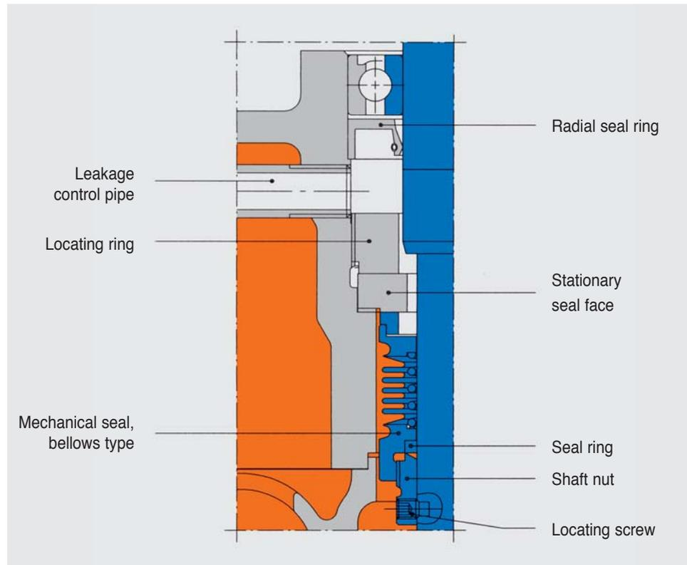
The rotating mechanical seal is fitted to the pump shaft by the shaft nut and the static seal ring. The stationary seal face is fitted to the bearing housing and sealed against the atmosphere by a gasket. The drive motor is protected against mechanical seal leakage by the grease lubricated radial seal ring. Seal leakage can be monitored by the leakage control pipe which is screwed to the bearing housing.
