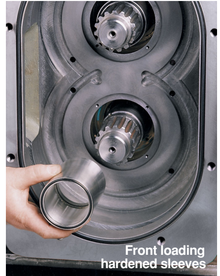
Replaceable restriction bushings
