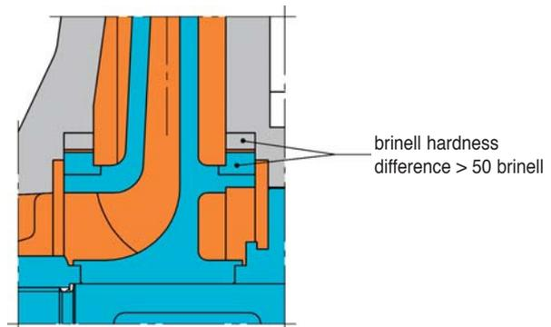
Mating wear surface materials have a difference in Brinell hardness of at least 50 HB.
